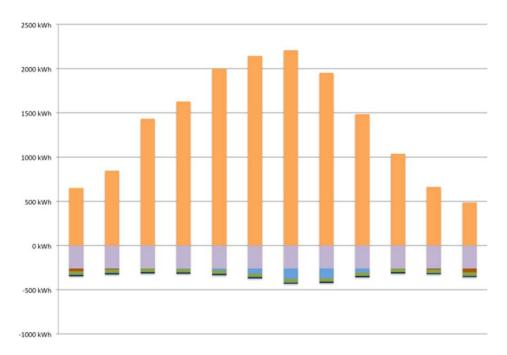
Figure 3 Overall energy consumption (negative scale) and production (positive) for Madrid from Jan to Dec..
