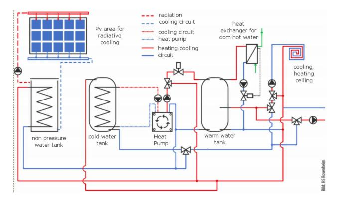
Figure 4 Schematic drawing of the mechanical services for heating, cooling and domestic hot water
