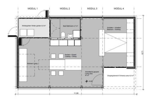
Figure 1 Floor plan and module structure
